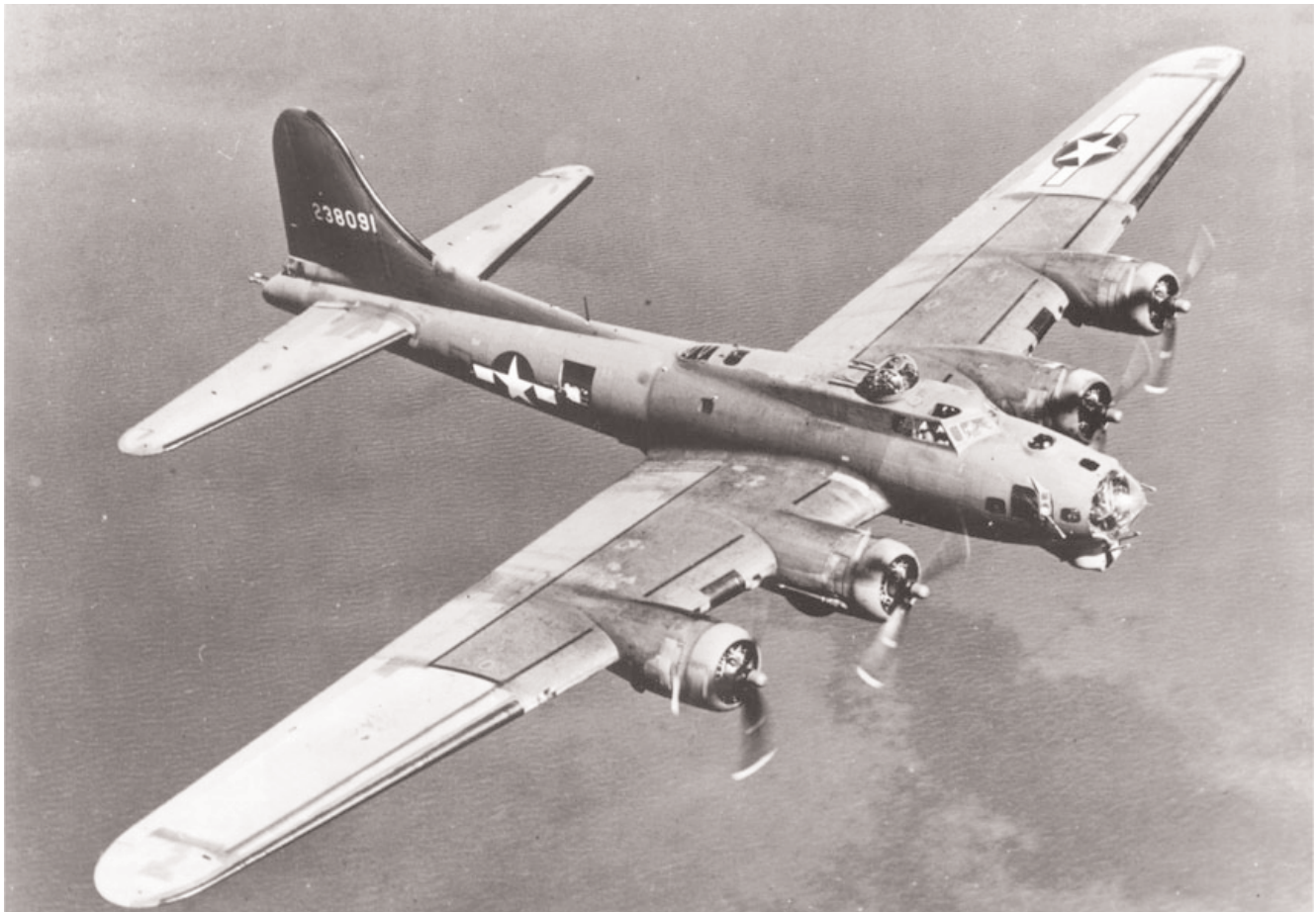
B-17 Flying Fortress bomber, showing the gunner turrets on top, in the nose, and in the tail.
