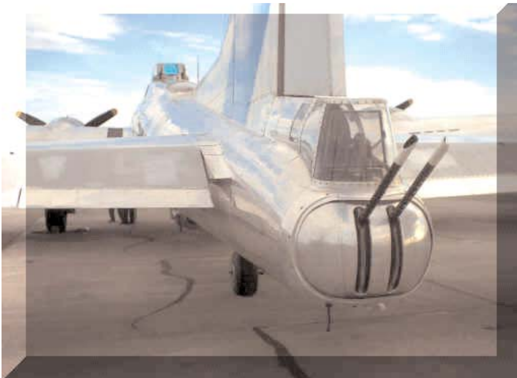
Picture of a B-17 Bomber Tailgun. A gunner sat inside the tailgun and shot at enemy aircraft.
